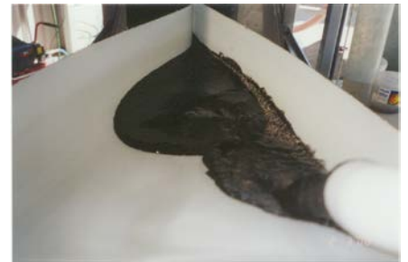
Slurry entering feed cavity
