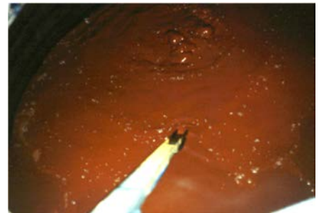
Feed slurry (air mixing)
